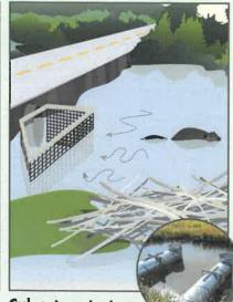
Culvert protectors prevent plugged culverts that can cause flooding of roads and other areas.
