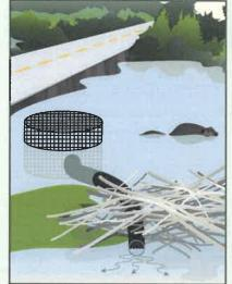
**Pond levellers** mitigate flooding by acting as an overflow valve through a beaver dam, allowing for the pond level to be managed at a level that prevents flooding but allows beavers to maintain their pond and habitat.
